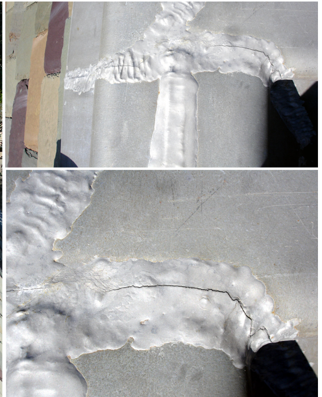
G16: close up of cracked solder joint
